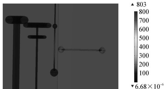
图13 均压球对垂直管母放电的电场仿真 Fig. 13 Electric field simulation of grading sphere to the vertical tube bus
